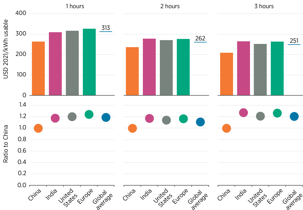
Figure 1.13 Turnkey battery storage system prices by market and duration, 2021
