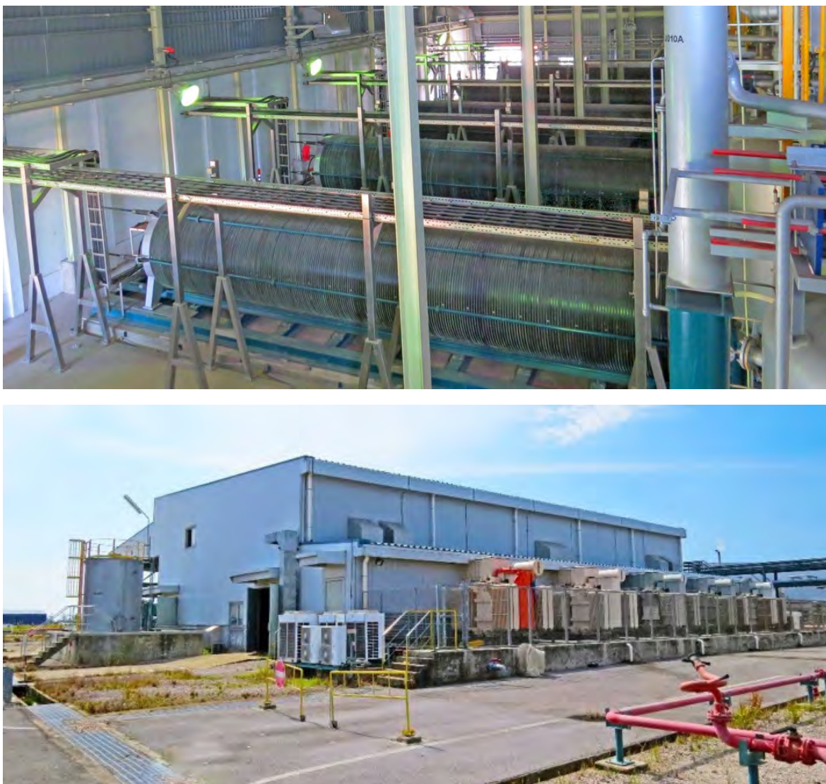
FIGURE 2.4 World's largest current electrolyzer (25 MW), polysilicon plant, Sarawak, Malaysia
