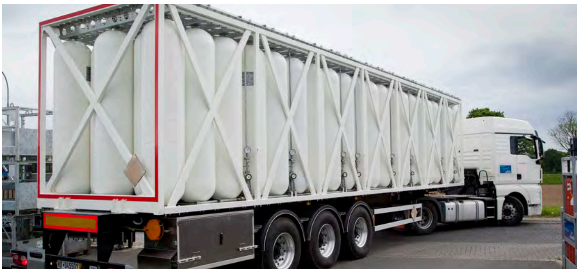
FIGURE 7.5 Pressurized hydrogen storage trailers
